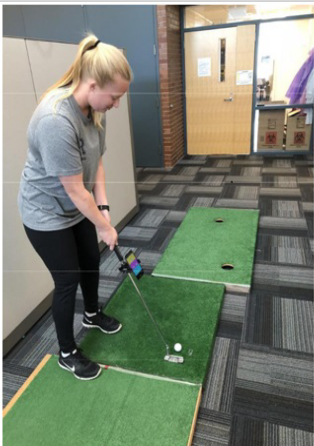
Figure 1: Experimental setup showing smartphone attached to the putter shaft and subject preparing to putt the ball to a hole (the further distance one) 6 ft away.
